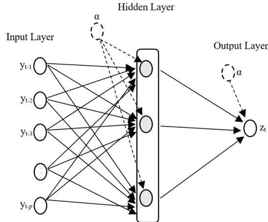
Figure 1 Artificial neural network's layers
